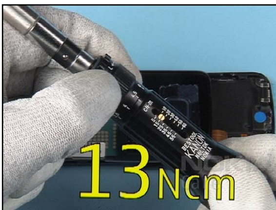
34. Set the correct torque.
