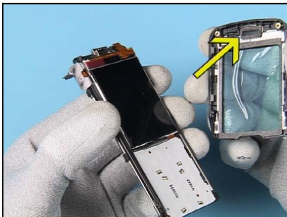
14. Mind the glued in earpiece gasket of the DISPLAY COVER.
