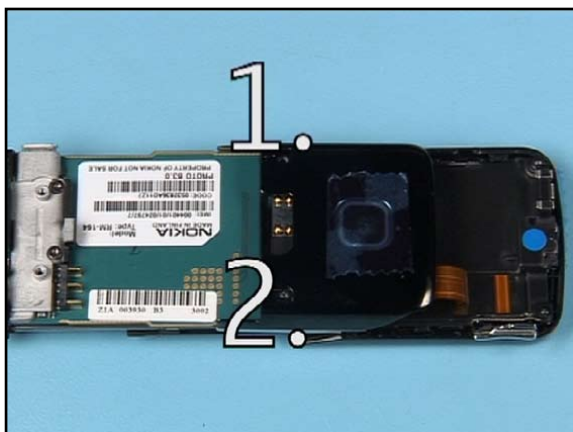
35. Apply the torque to the screws in the order shown.
