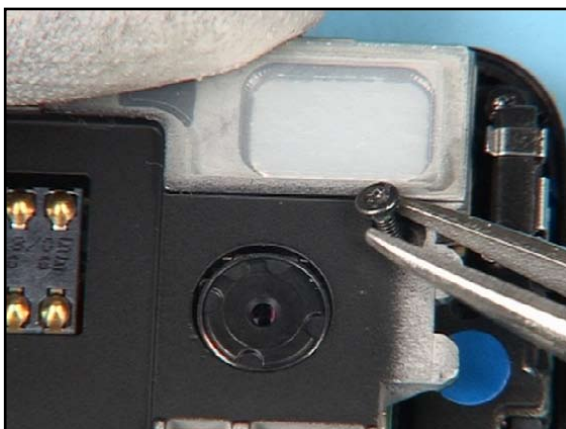
28. Insert 6 new screws.
