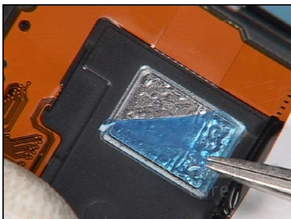
9. Peel up this protective film if this part was renewed.
