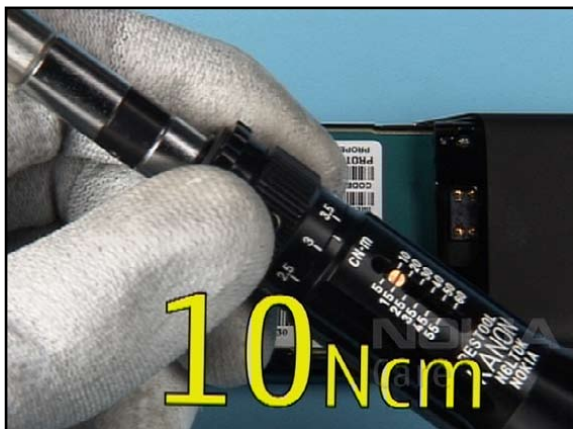
47. Set the correct torque.
