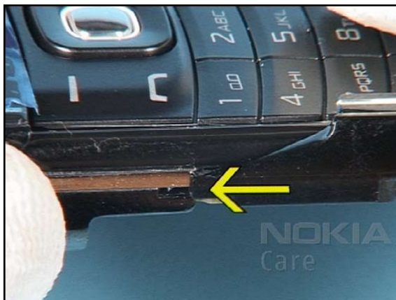
44. Nopte the correct positioning of these clips before going on.
