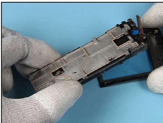
28. The DISPLAY COVER can be separated now.
