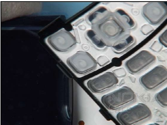
9. This BLACK KEYPAD can be reused if the adhesive stays on the keypad. Otherwise it must be renewed when reassembling.
