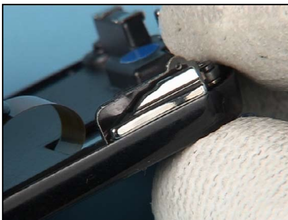
36. Do not forget fitting the VOLUME KEY ASSEMBLY.
