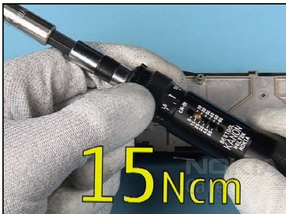
19. Set the correct torque.
