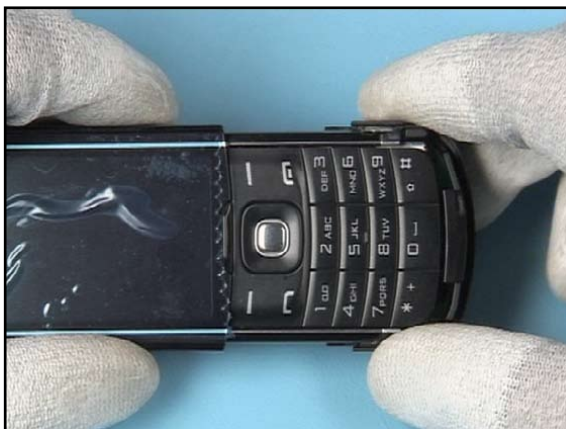
42. Check the positioning of the BLACK KEYPAD before going on.
