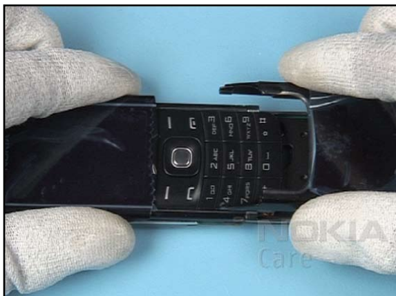
43. Click the snaps of the KEYPAD COVER ASSEMBLY into their places.
