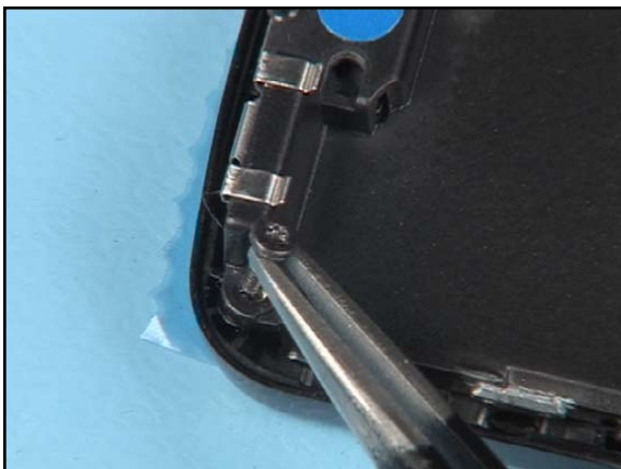
18. Insert 2 new screws.
