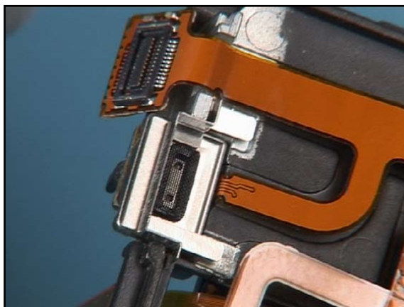
8. Place the EARPIECE ASSEMBLY.
