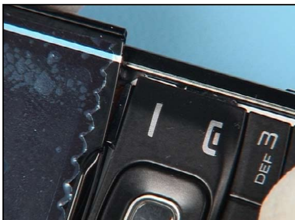
39. Insert the snaps of the BLACK KEYPAD at the shown side first.
