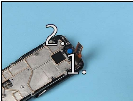
26. Unscrew these 2 Torx Plus size 4 screws in the order shown and remove them.
