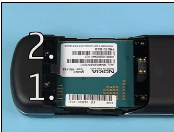
48. Apply the torque to the screws in the order shown.
