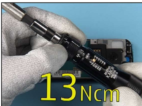
29. Set the correct torque.
